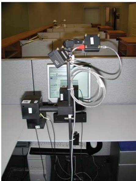
Figure 2: Interior photos of newly constructed testbed for New York Times building. At left, view toward the west façade, with two different shade systems partially deployed. At right, an instrumentation cluster at a workstation, including illuminance and luminance mapping sensors, and a webcam.
