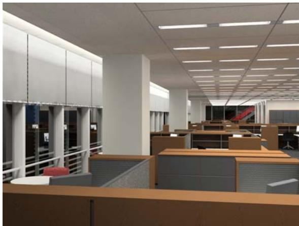
Figure 3: Initial RADIANCE simulations of the west façade of the New York Times building. Left: Without interior automated shading, the exterior ceramic rod shading system is insufficient to control glare on work surfaces. Right: A night view of a more refined image with actual furniture layout, electric lights on, with shades partially deployed.
