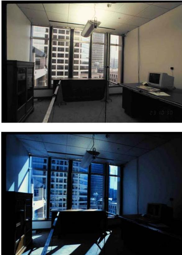
Figure 4: Electrochromic test rooms in Oakland, CA. The room at left is in a clear transmission state on an overcast morning; at right the sun has emerged and the window switches to its darkest state to control glare at the computer workstation.
