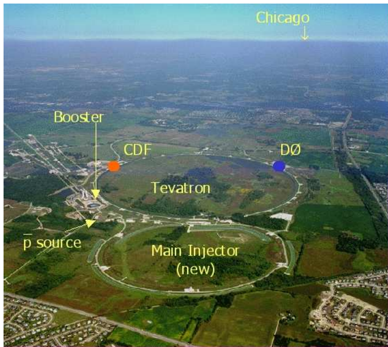
Figure B.1: (a) A schematic of the Fermilab accelerator chain. (b) An aerial photograph of Fermilab. For a sense of scale the Main Injector is one kilometer in diameter and the Tevatron is two kilometers in diameter.
