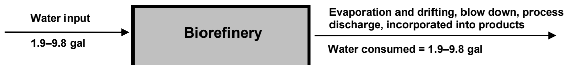
FIGURE 21 Water Input and Consumption for a Biorefinery Producing One Gallon of Cellulosic Ethanol (water recycle may occur)
