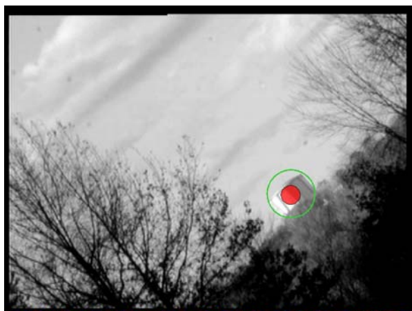
Figure 39. Water tower as viewed by transceiver video camera. The telescope ocular field of view is illustrated by the green circle. The smaller circle is the approximate footprint of the laser beam.
