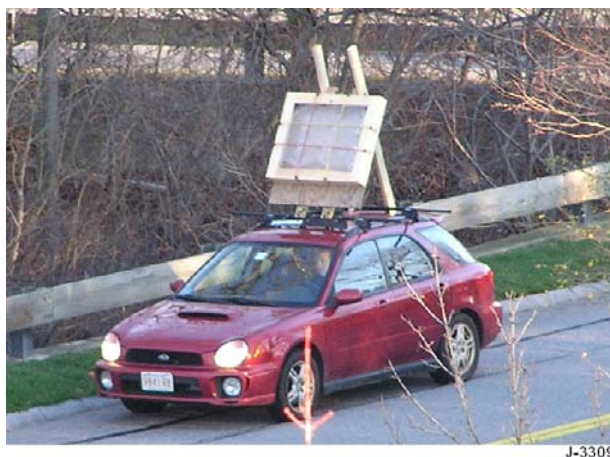
Figure 50. Methane target assembly mounted to the roof of an automobile.
