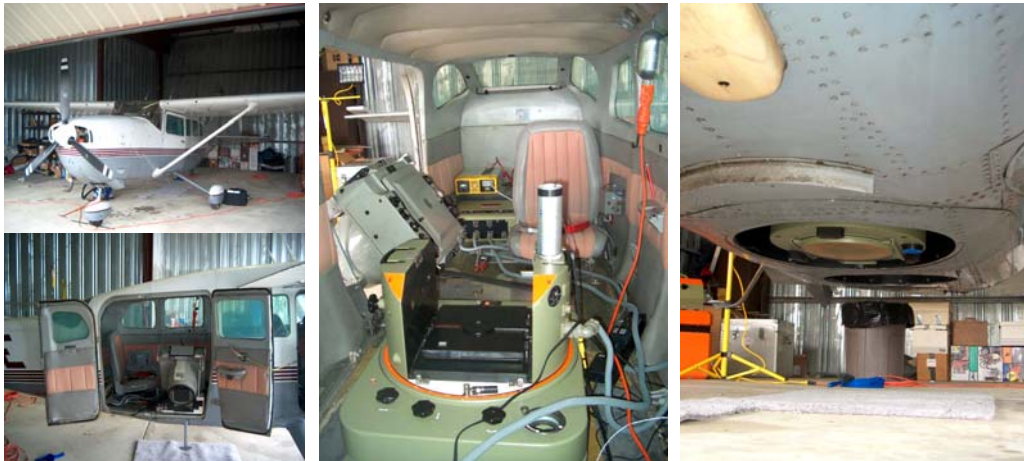
Figure 1. Gamm Air's Cessna 207, cabin with photographic equipment installed, and exterior view of camera port.
