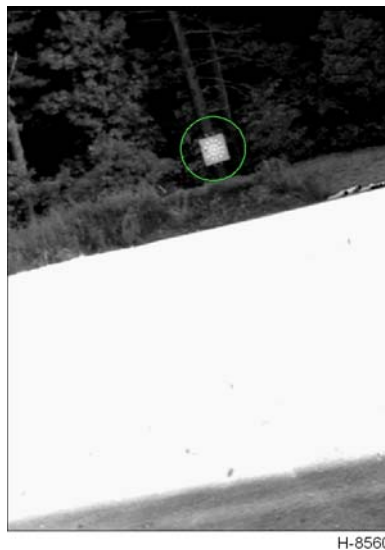
Figure 31. Camera view of plywood target with retroreflective tape at 200m range. Telescope ocular field of view is illustrated by the green circle.
