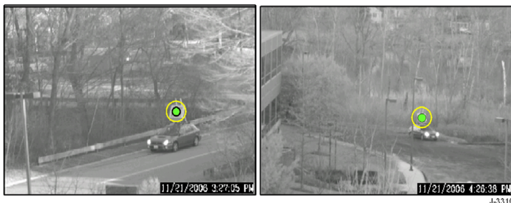
Figure 51. Recorded camera images from simulated flight test experiments at 115\text{m} range (left) and 185\text{m} range (right). Again, the telescope ocular field of view and laser footprint are indicated.
