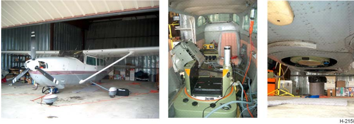
Figure 7. Gamm Air's Cessna 207, cabin with photographic equipment installed, and exterior view of camera port
