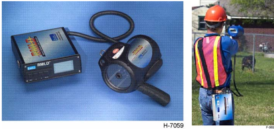
Figure 1. Photographs of PSI's remote methane leak detector (RMLD) production version (left) and advanced prototype during field testing (right).
