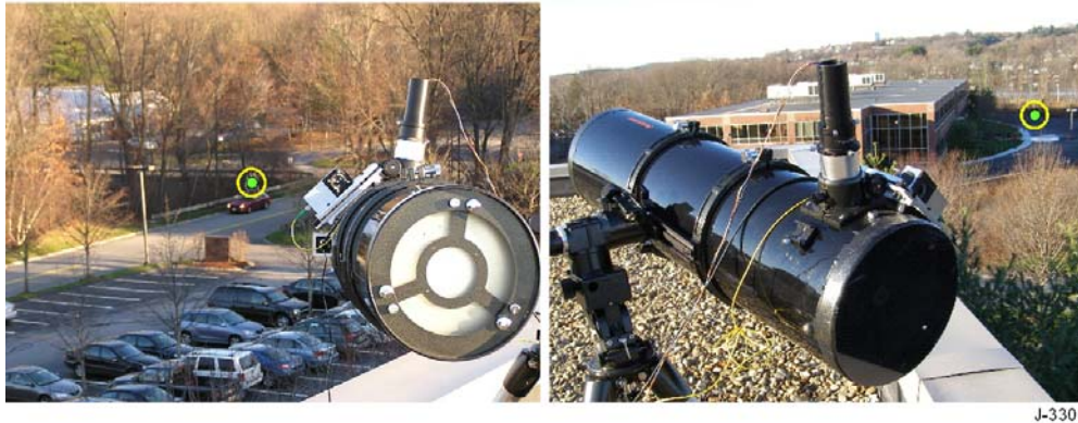
Figure 49. View from sensor transceiver to measurement location for the 115m path (left) and 185m path (right). Yellow circles indicate approximate telescope field of view and green circle indicates approximate laser footprint.
