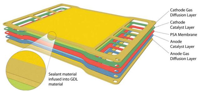
Figure 1. Schematic of a typical MEA
