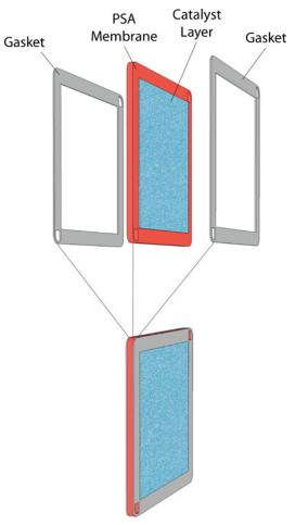
Figure 11. Thin-strip sealing zone of the CCM
