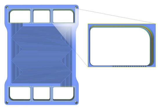
Figure 14. Schematic of cell misalignment in cell stack
