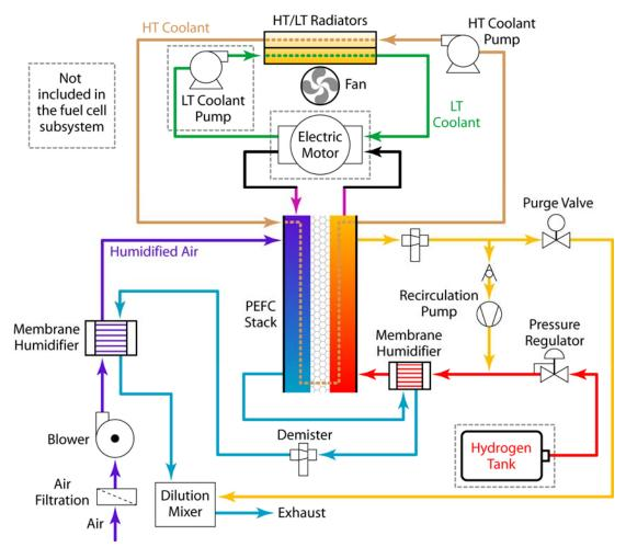
Figure 19. Alternative diagram of atmospheric PEM fuel cell system
