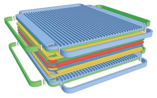
Figure 6. Cell stack with a combination internal-external manifold
