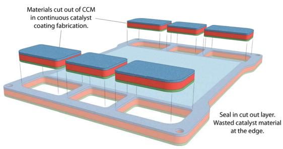
3. Bond the catalyst-coated membrane to a prefabricated manifold.
