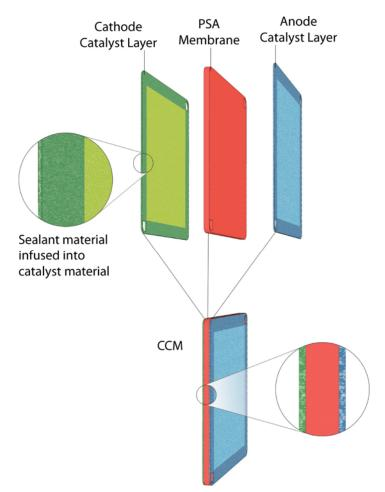
Figure 3. Decal transfer of the catalyst layer by hot pressing or hot roll pressing is used to transfer the preformed catalyst layer onto the PSA membrane.
