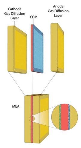
Figure 2. The carbon felt, carbon paper, or graphite cloth are bonded to the CCM using a seal around the edges of the gas diffusion layer.
