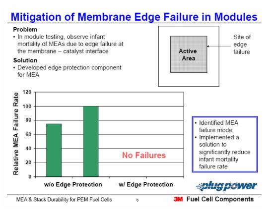
Figure 15: Edge seal protection<sup>6</sup>
