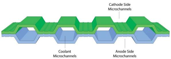
Figure 13. Cross section of metallic bipolar plate showing contacts to adjacent cells.
