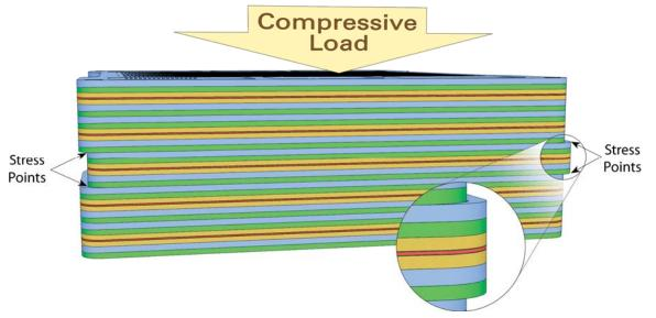
Figure 17. Seals are designed to have height and compressive properties that assure the GDLs, the catalyst layers, and the membranes remain in contact for water/proton transport.
