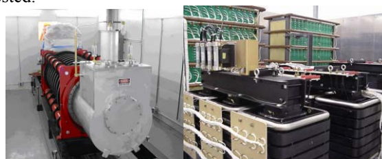
Figure 1: a. (left) the CPI klystron. b. (right) the 95kV 20A DRC power supply.
