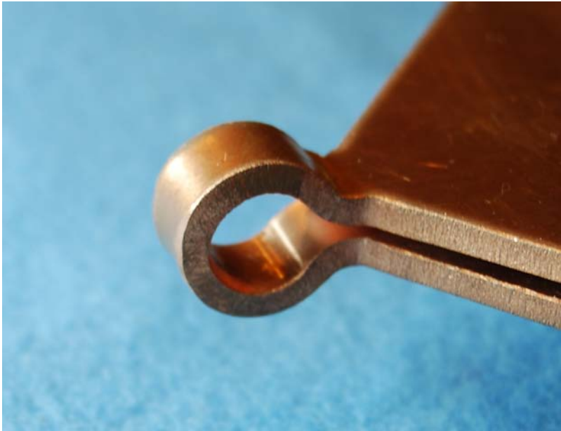
Fig. 2. Two-megagauss single-turn coil design, courtesy C. Mielke, LANL.
