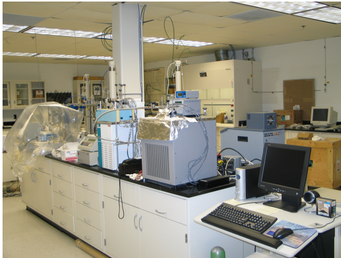
Figure 2. High-pressure manometric/volumetric setup used in this study, including the dry nitrogen positive flow glove bag, the constant temperature bath, the syringe pump, and the CO 2 gas cylinder.
