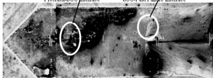
SEM micrographs of DCB specimens with 0.5 wt% Si subjected to SCC testing at 100°C in acidic solution for 30 days
