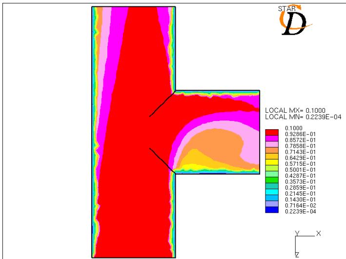
Concentration profile for T-joint at Re = 200,000 .
