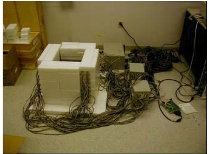
Neutron Multiplicity Detector System configured in a cubic geometry for background and source counting.
