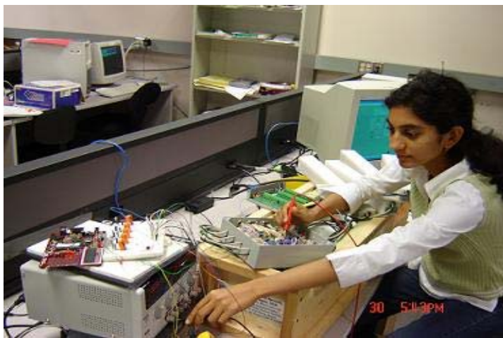
Graduate student Shrutti Patil checks signals on one of the 8-detector control boxes of the NMDS.
