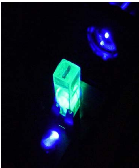
Laser induced fluorescence of a uranium sample in nitric acid
