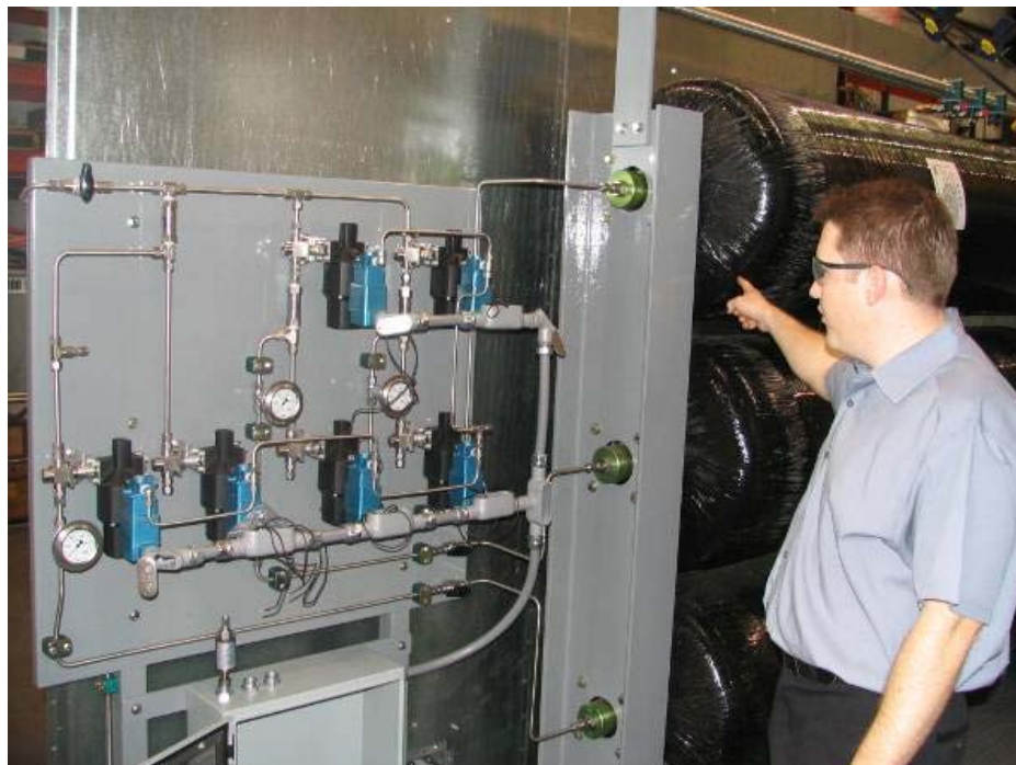
Figure 29: Factory-Packaged, Transportable Hydrogen Station Cascade
