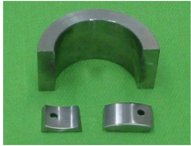
Figure 1 – Section of 12 (10.5Cr) pipe (2-in O.D.) and curvature samples cut from pipe. All but one side of the curvature samples are flat. Samples: concave (left) and convex (right).
