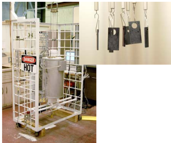
Figure 4 – Cyclic oxidation apparatus for testing in atmospheric pressure steam/air mixtures at up to 800°C.
