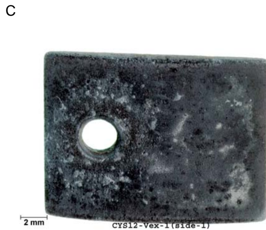
Figure 12 – A) Cyclic oxidation results for concave and convex 12 (10.5 Cr) at 760°C in 50% H 2 O-50% air with hourly cycles. B) Light microscopy for concave 10.5 Cr after 2000 hr. C) Light microscopy for convex 10.5 Cr after 2000 hr.
