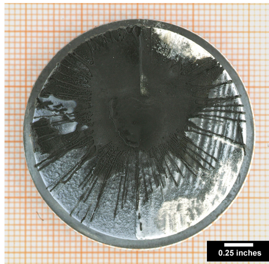
Figure 1. Post-rocket test photograph of a graphitic test specimen that had a protective coating applied to one-half of its surface (right side of the picture).
