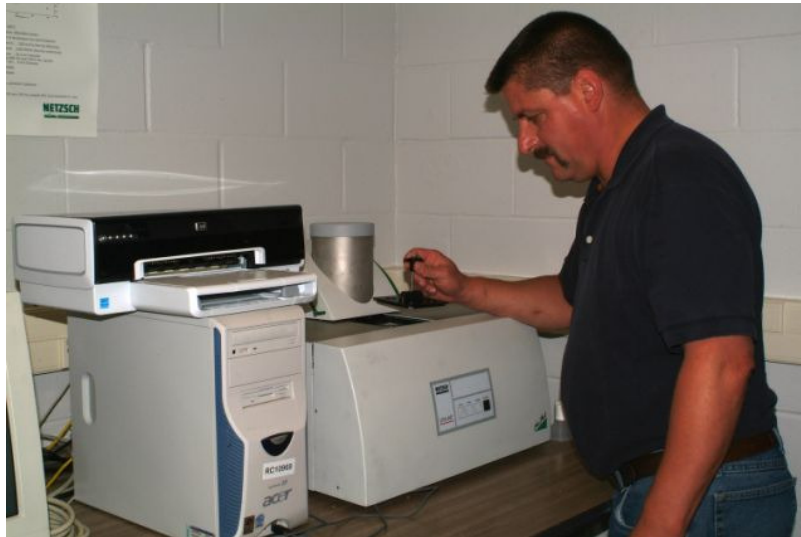
Figure 7. LFA 447 Thermal Diffusivity unit being loaded.
