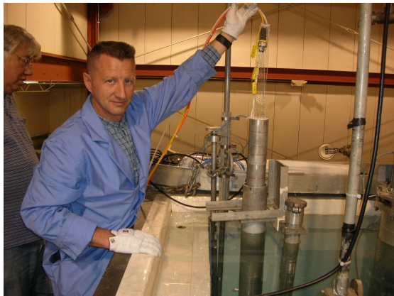
Figure 1. (Left) Ta-10W and T-111 test specimens were placed within cadmium wrapped tube furnace prior to loading within reactor test pipe. (Right) Reactor core at bottom of water pool (middle of photograph) at Ohio State University.
