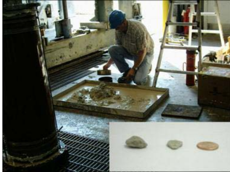
Figure 7-1. Cuttings from drilling tests (Left: roller cone; Middle: hammer underbalance; Right: penny coin)
