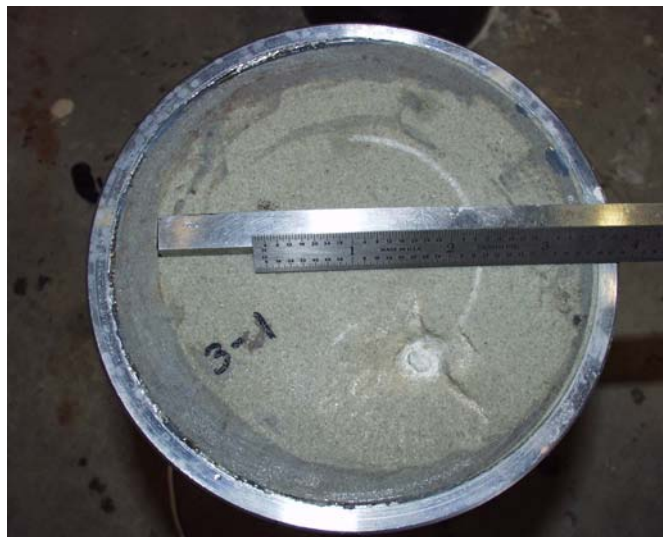
Figure 6-6. Top view of impacted Berea sandstone specimen
