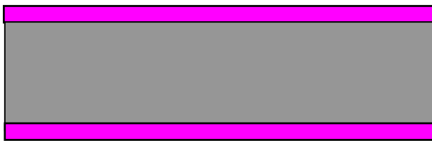
(a) Sub-atmospheric CVD to form 1.0 \mu\text{m} low stress nitride (LSN).
