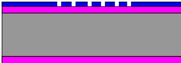
(b) Chromium deposition and patterning the isolation trenches to form the connection wires and the switching electrodes
