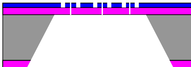
(d) Pattern the backside window into LSN layer and etch through the silicon wafer in KOH.
