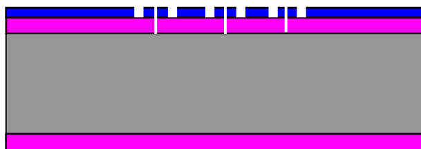
(c) Pattern the switching apertures through the chromium layer and the silicon nitride layer using chromium wet etch process and silicon nitride plasma etch.
