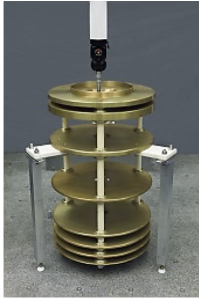
Figure 2.4. Parallelism and concentricity inspection. 1
