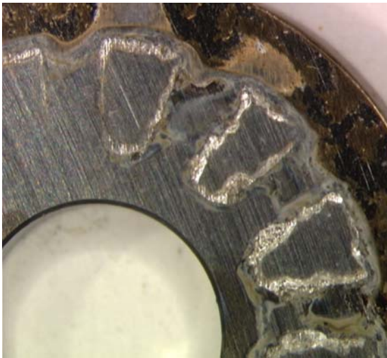
Figure 4.11 – Specimen JE3328, MA polished Alloy 22 after CPP in 1 M NaCl at 90°C
