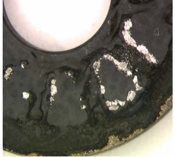
Figure 4.18 – Specimen JE3373, SHT Alloy 22 after CPP in 0.1 m NaCl + 0.001 m NaHCO 3 at 95°C
