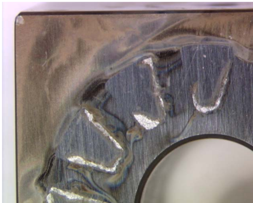
Figure 3.5 - Alloy 22 Specimen AY009 after CPP in 1 M \text{NaCl} at 90°C showing Major Transpassivity in the bold areas. Crevice Corrosion under CF, Magnification ~X 8
