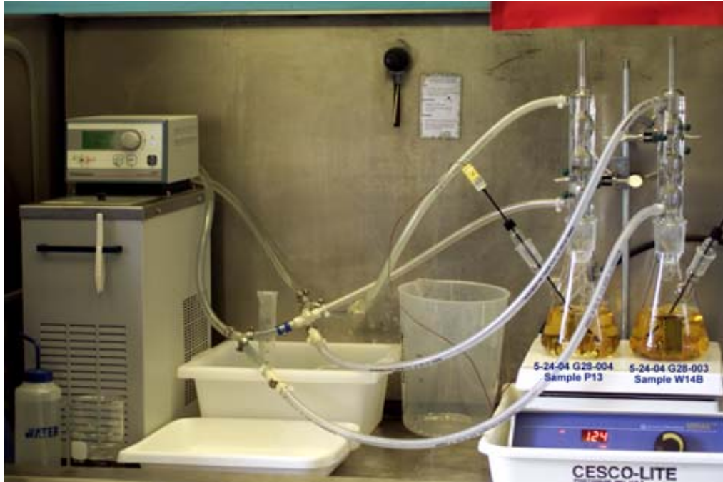
Figure 5.1 - Set-up for immersion corrosion testing
