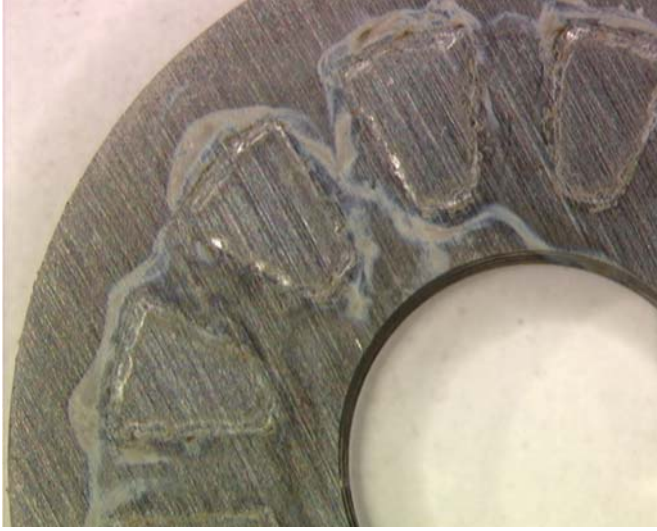
Figure 4.17 – Specimen JE3381, MA polished Alloy 22 after CPP in 0.1 m NaCl + 0.001 m NaHCO 3 at 95°C
