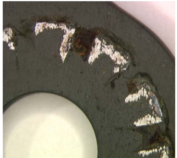
FIGURE 4.12 – Specimen JE3303, SHT Alloy 22 after CPP in 1 M NaCl at 90°C
