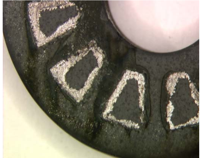
Figure 4.14 – Specimen JE3308, SHT Alloy 22 after CPP in 6 m NaCl + 0.3 m KNO 3 at 100°C
