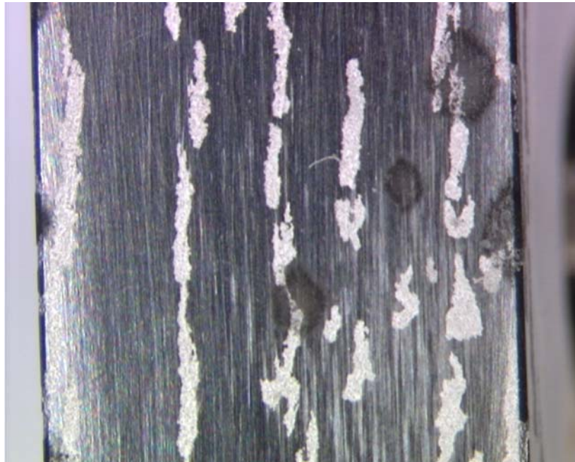
Figure 3.4 - Alloy 22 Specimen AY011 after CPP in 12 m \text{CaCl}_2 + 6 m \text{Ca}(\text{NO}_3)_2 at 130°C showing Localized Attack on the ST Face (non-creviced), Magnification ~X 8
