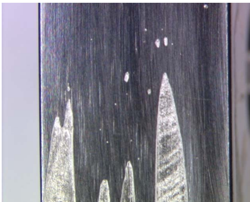
Figure 3.2 - Alloy 22 Specimen AY008 after CPP testing in 5 M \text{CaCl}_2 at 90^\circ\text{C} showing Typical Massive Localized Attack on the ST, Non-Creviced Face
