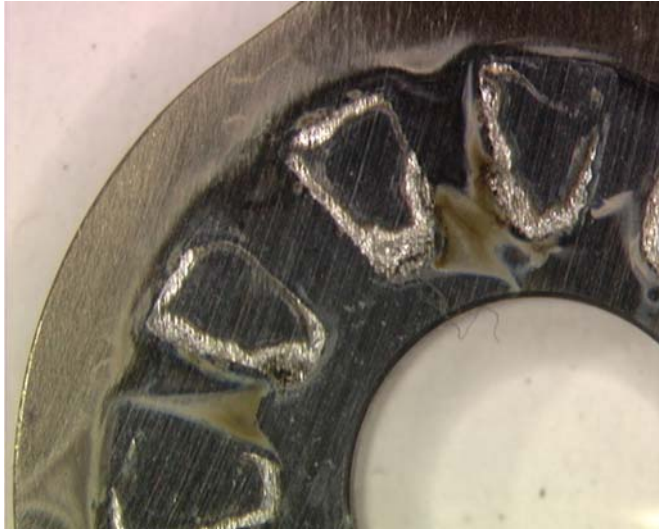
FIGURE 4.13 – Specimen JE3315, MA Alloy 22 after CPP in 6 m NaCl + 0.3 m KNO 3 at 100°C
