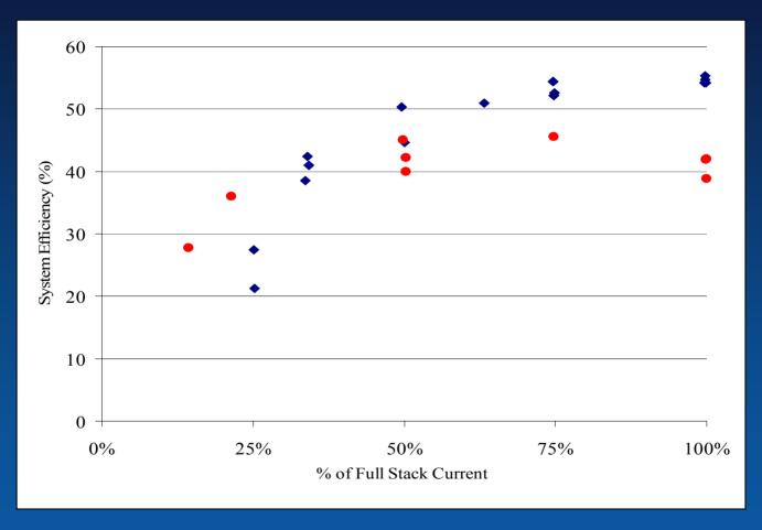
• System efficiency of PEM system at various levels of current and temperature
