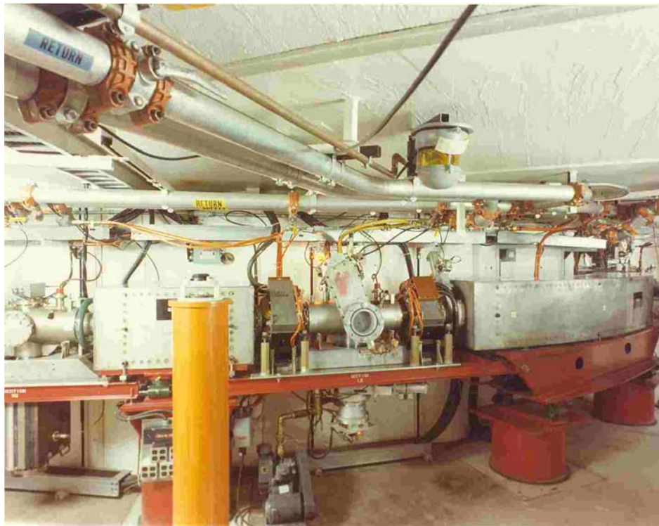
Fig 1. View inside the Rapid Cycling Synchrotron enclosure. On the right is a triplet main ring magnet. On the left, behind the survey post, is a singlet main ring magnet.
