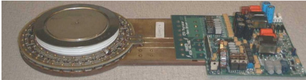
Fig. 4.10. 4000-A/4500-V ETO with the integrated gate driver [9].
