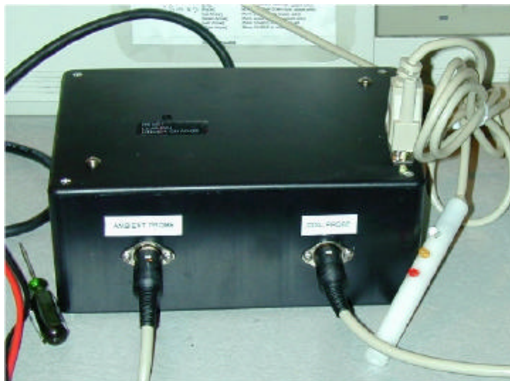
Fig. 1. Pre-prototype charge indicator with analog technology
