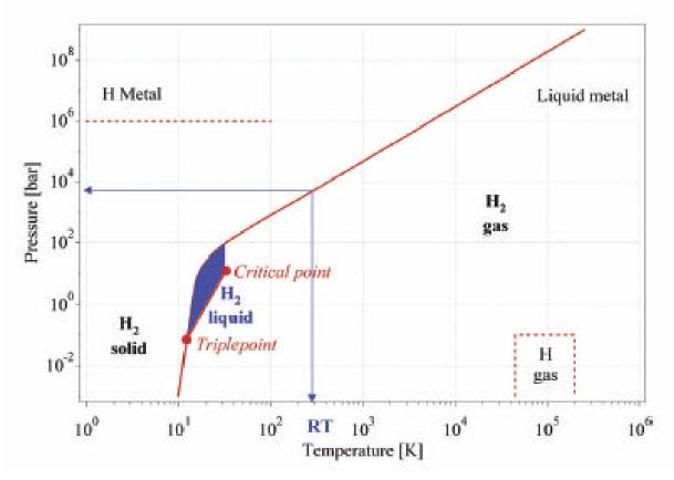
Liquid hydrogen only exists between the solid line and the line from the triple point at 21.2 K and the critical point at 32 K.
