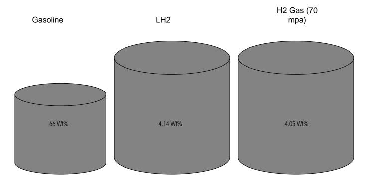
Calculation of the gravimetric energy density of fuel needed to drive 250 miles. Expressed as a percentage of the weight of fuel to the weight of fuel storage system
