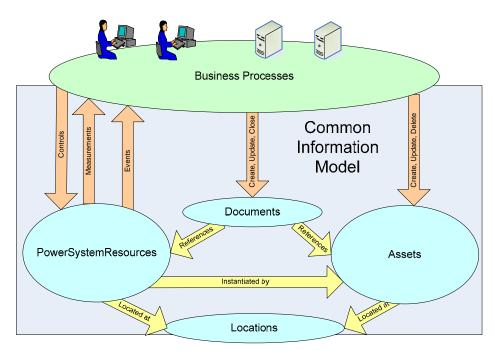
Electrical transmission and distribution networks are modeled in terms of Power System Resources. Power System Resources are logical entities that typically correspond to physical Assets. Business processes may control and monitor power system resources. Central to most business processes is the notion of a 'document' as a unit of information exchange, where a document typically contains references to Power System Resources and/or Assets.
