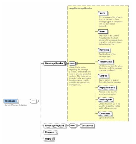
As a partial answer to this issue, the IEC 61968 standard for XML-based information exchange will factor the out separate header and payload message sections. The message header contains a verb, identifying a generic action, and a noun identifying the type of the payload.
