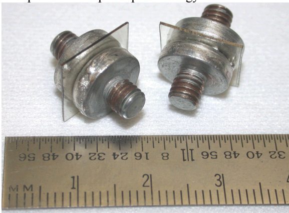
Figure 2. Vanadium compensated, semi-insulating, 6H-SiC PCSS assembly.
