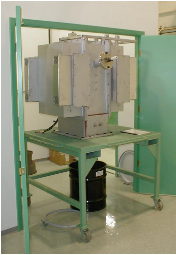
Figure 7a: Furnace and cart for dripping molten slag on a test refractory brick. The spent slag is collected in the black barrel below the cart. The slag feed tube protrudes from the front of the upper part of the furnace. The slag feeder is not shown.
