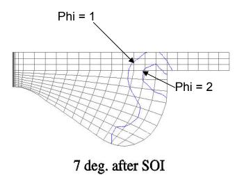
Fig. 5 Predicted fuel/air equivalence ratio contours for SOI -18 ATDC at the experimental start of combustion time
