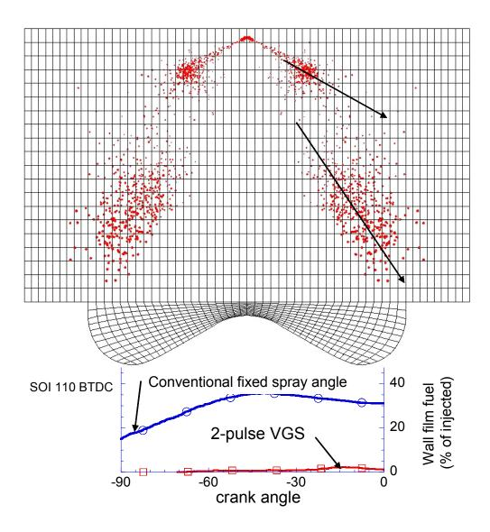
Figure 2. Optimized spray angle in each injection pulse gives improved fuel-air mixing, and significantly reduced impinged fuel during the compression and combustion processes
