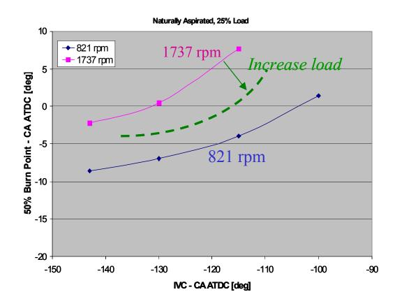
Figure 1. Combustion phasing control with variable valve timing. 50% burn point versus IVC for different engine speeds and loads.
