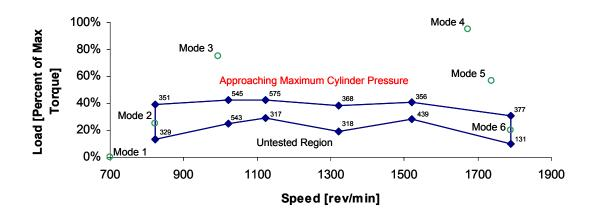
Figure 2 Early start-of-injection operating regime for PCCI combustion
