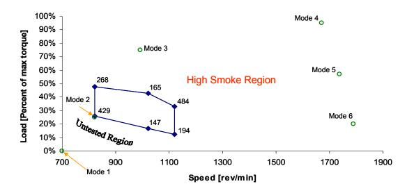
Figure 1 Late start-of-injection operating regime for PCCI combustion
