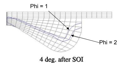
Fig. 4 Predicted fuel/air equivalence ratio contours for SOI –9 ATDC at the experimental start of combustion time
