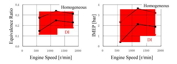
Figure 4. HCCI operating ranges for complete homogeneous charge mixtures and the optimum combination of premixed and direct injected fuel. CR = 16.55, Fuel = PRF 92, Tintake = 107 °C.
