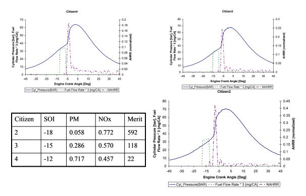
Fig. 3 Measured cylinder pressure, heat release rate and fuel injection rate as a function of start of injection timing for early injection cases
