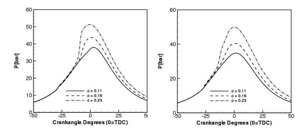
Figure 6. Computed (left) and measured (right) in-cylinder pressure with variations in equivalence ratio  $\Phi$  for premixed n-heptane/air in the CFR engine. From Ref. [18].
