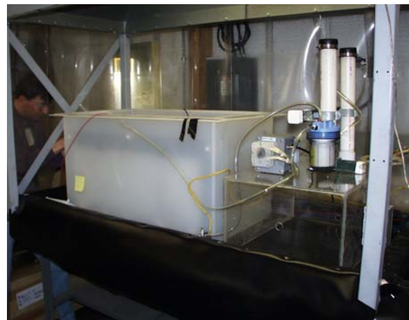
Figure 10 EKAR cell. Pump, filter, and ion exchange columns are at right.
