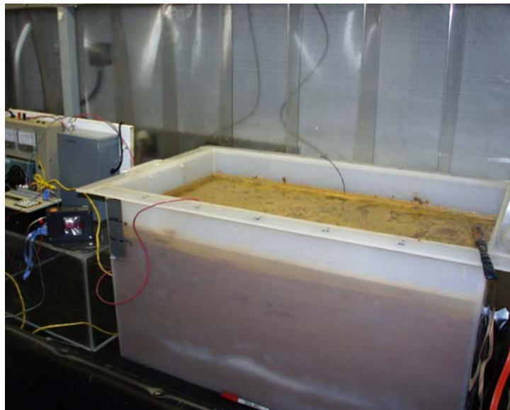
Figure 7 Filled ECRTs cell. Power supply and datalogger shown at left.
