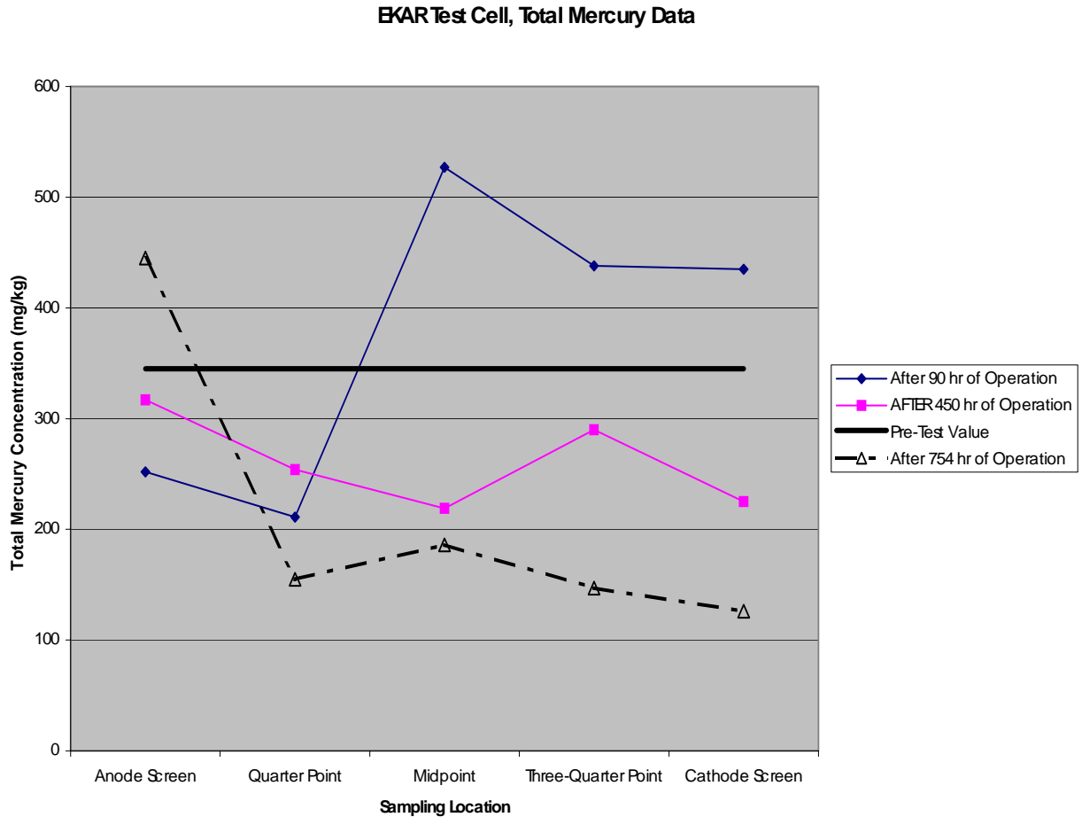
Figure 18 EKAR Test Cell Pre-test and after 90 hr, 450 hr and 754 hr of Operation Total Mercury Distributions
