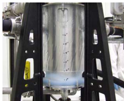
Fig.3. Mixing Annulus in V-05, 2L/min.
