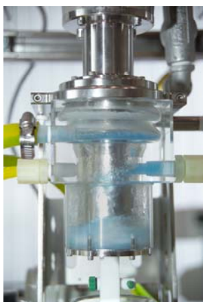
Fig. 2. 5 cm Clear Housing Contactor View
