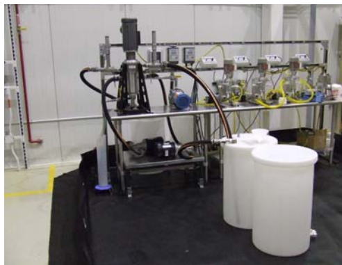
Fig 1. Centrifugal contactor test assembly
