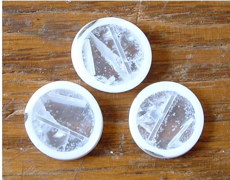
Figure 8.1. Slices of crucibles with sapphire and zirconia in soda lime glass.
