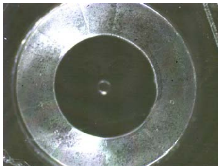
Figure 3.14. Ferrule and diaphragm bonded with ring.
