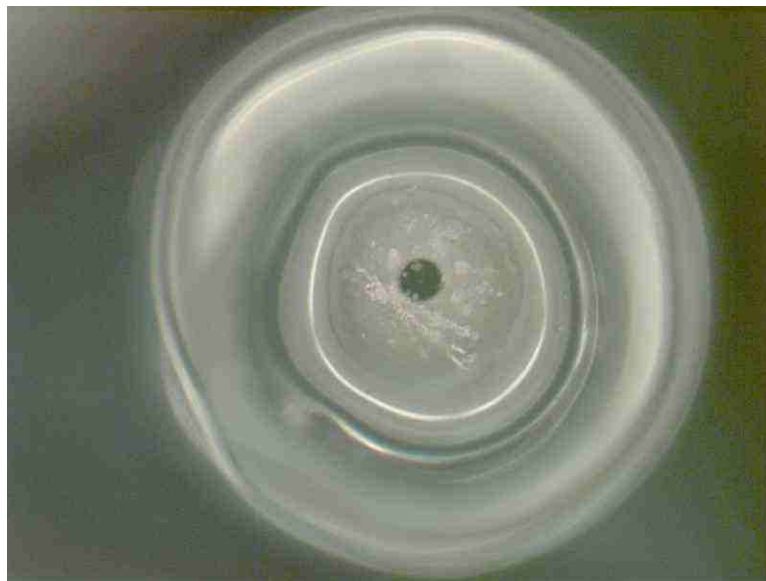
Figure 3.59. Micrograph of diaphragm and ferrule laser bonding (top view).
