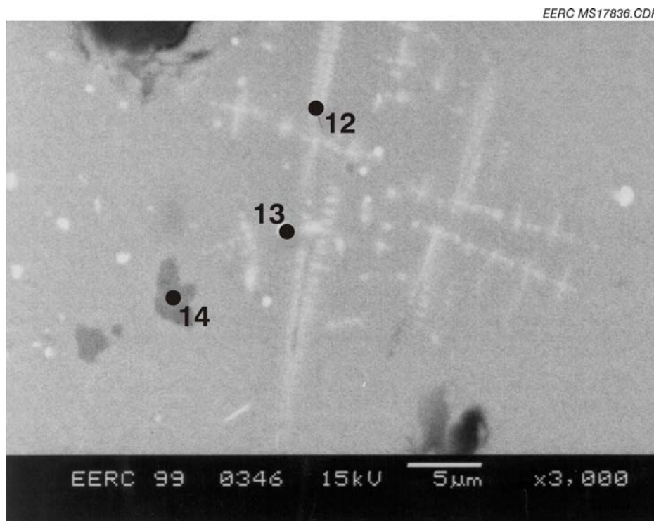
Figure 28. SEM micrograph of mixing zone deposit from gasification Test P061 on Tuscaloosa petcoke showing Points 12–14.
