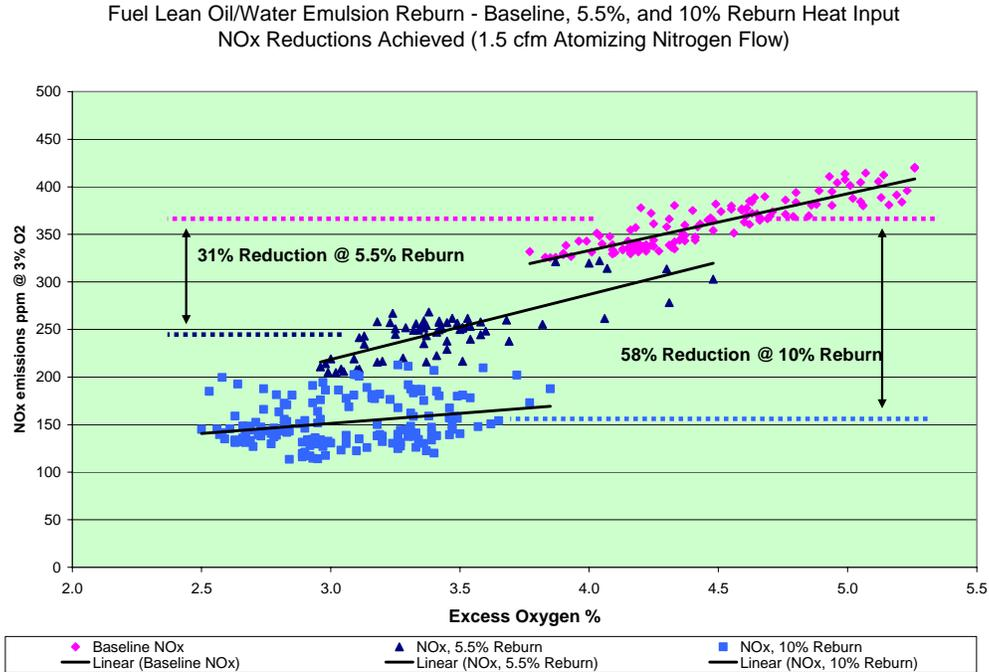
**Figure 9. Fuel Oil/Water Emulsion Reburn Results at 10% Reburn Fuel Heat Input**
