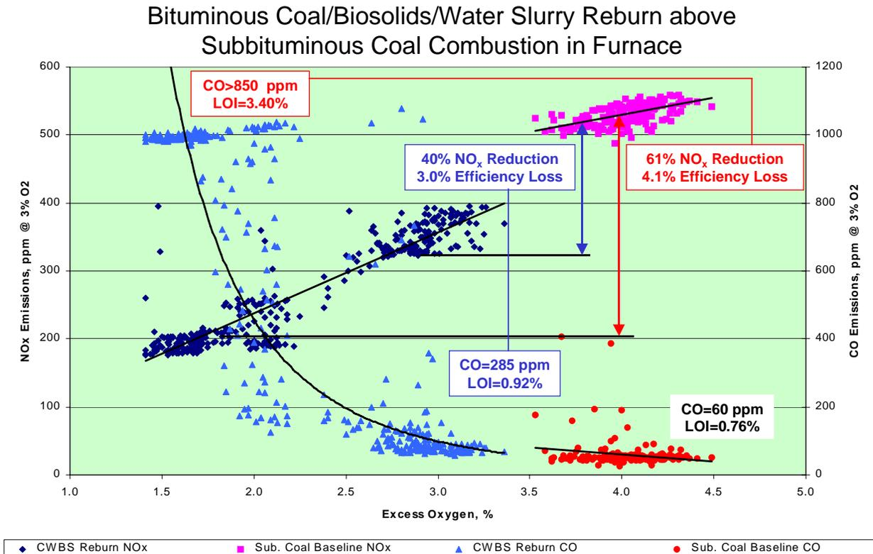
**Figure 6. Coal/Water/Biosolids Slurry Reburn Results**
