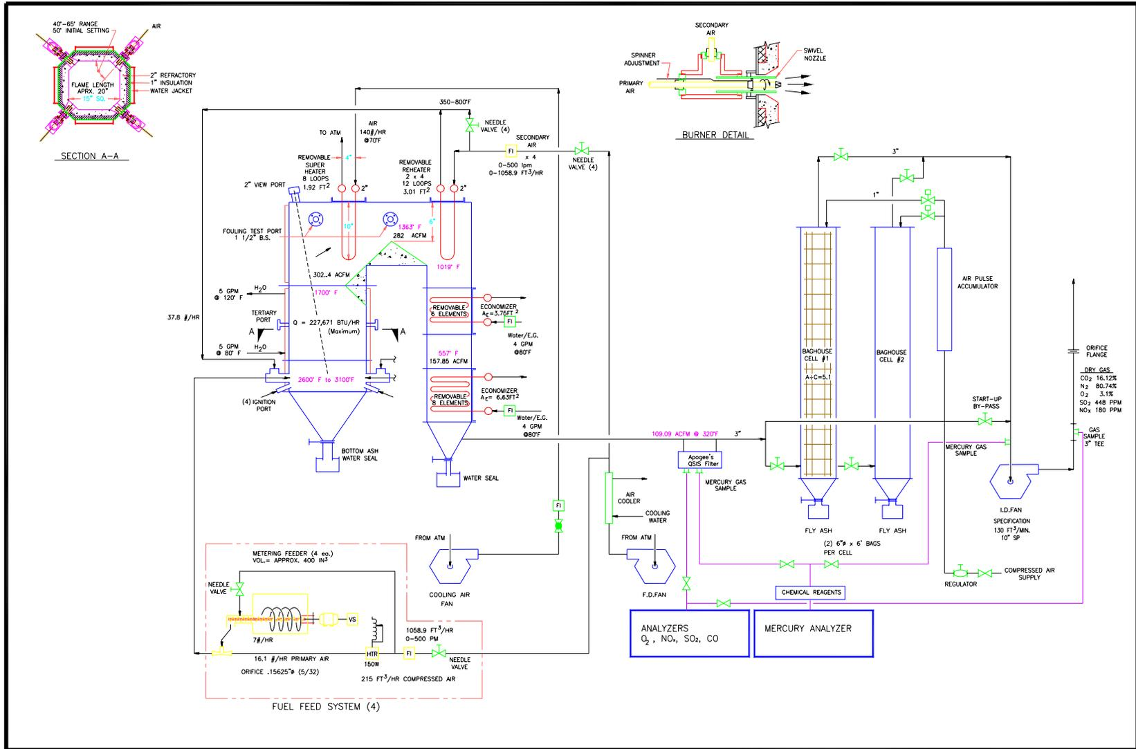
Figure 4. A Schematic of the CTF
