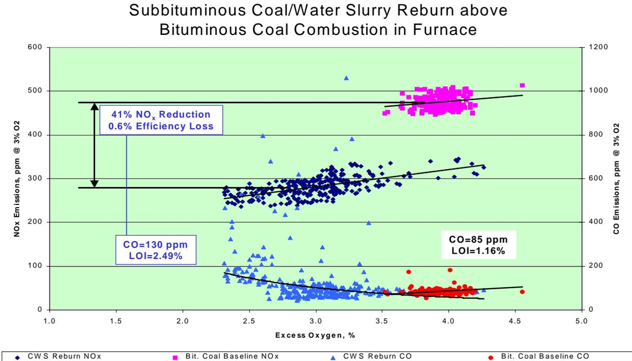
**Figure 7. Coal/Water Slurry Reburn Results**
