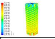
Figure 1: Computational model of an eight-fin helical channel heat exchanger.
