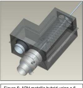
Figure 5: APH metallic hybrid using a 6 fin ceramic heat exchanger element
