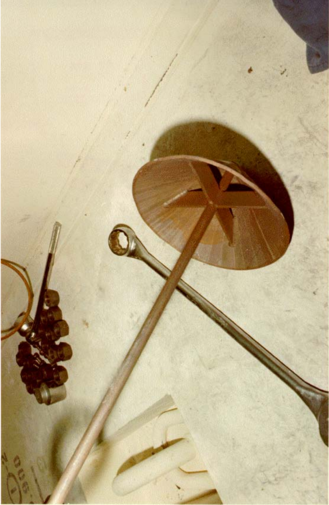
Figure B-4. View of the Calciner baffle plate inspection plug following decontamination. The plug is free of calcine. Compare with Figure A-5 for the pre-decontamination condition of plug when it was filled with calcine (82-246).
