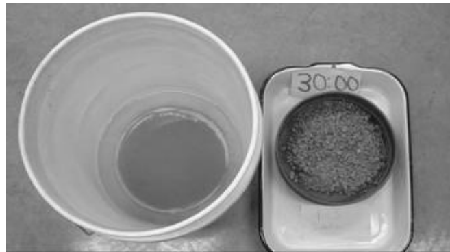
Figure 13: On the right is the Tyler 10 mesh screen holding the previously immersed agglomerates. The bucket on the left contains the fines which have been released due to the breakdown of the agglomerates.
