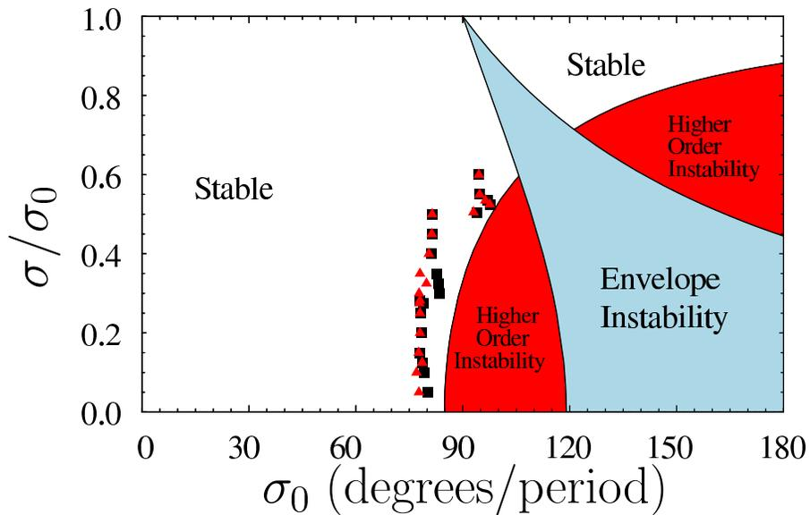
Fig. 5. (color online) Beam stability boundary calculated from a core-particle model for a FODO quadrupole channel. ( $L_p = 0.5$  m,  $\eta = 0.5$ ,  $\varepsilon = 50$  mm-mrad).
