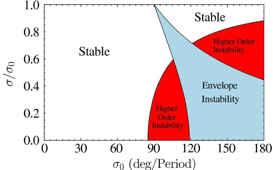
Fig. 1. (color online) Beam stability regions in a FODO quadrupole lattice.
