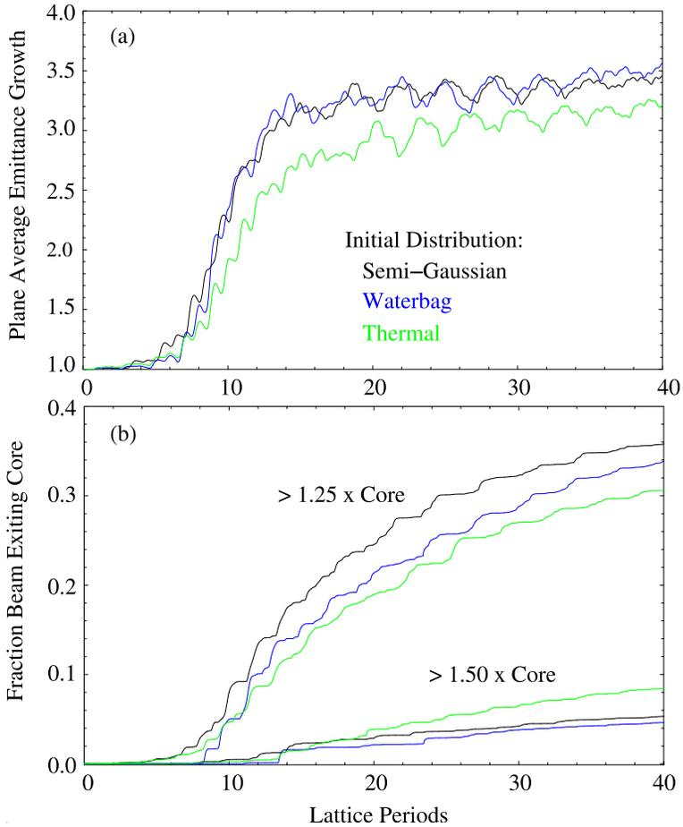
Fig. 2. (color online) PIC simulations of (a) the plane-averaged emittance growth for different initial distributions in a FODO quadrupole channel, and (b) the fraction of the beam distribution evolving outside the core. ( $\sigma_0 = 100^\circ$ ,  $\eta = 0.5$ ,  $L_p = 0.5$  m,  $\sigma/\sigma_0 = 0.2$ , and  $\varepsilon = 50$  mm-mrad).
