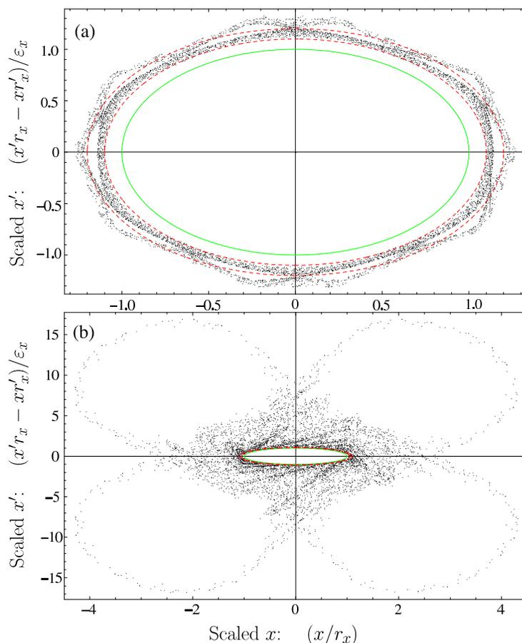
Fig. 4. (color online) Core-particle Poincaré phase-spaces for  $\sigma_0 = 100^\circ$ ,  $\sigma/\sigma_0 = 0.67$  (a), and  $\sigma/\sigma_0 = 0.2$  (b). ( $L_p = 0.5$  m,  $\eta = 0.5$ ,  $\varepsilon = 50$  mm-mrad).
