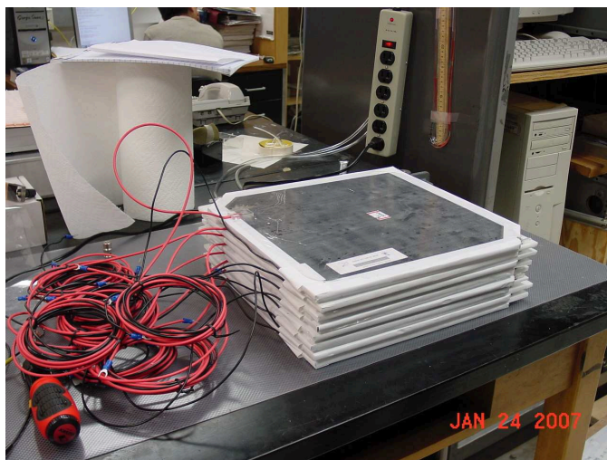
Figure 3.30: Shown are eight RPC gaps on arrival from Korea University at GSU in Atlanta. 5 gaps have been produced with the standard CMS oil coating; 3 gaps without and detailed comparisons of the performance of the different detector gaps will be carried out.
