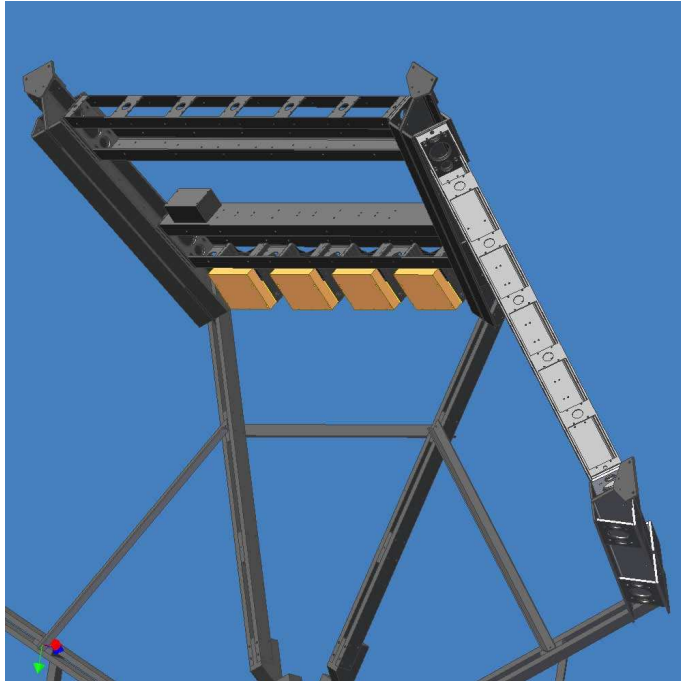
Figure 3.86: Location of station 2 new FEE. Yellow boxes are new FEEs which are piggy backed on the old FEE. The TX board is installed at the space indicated by the white arrow.
