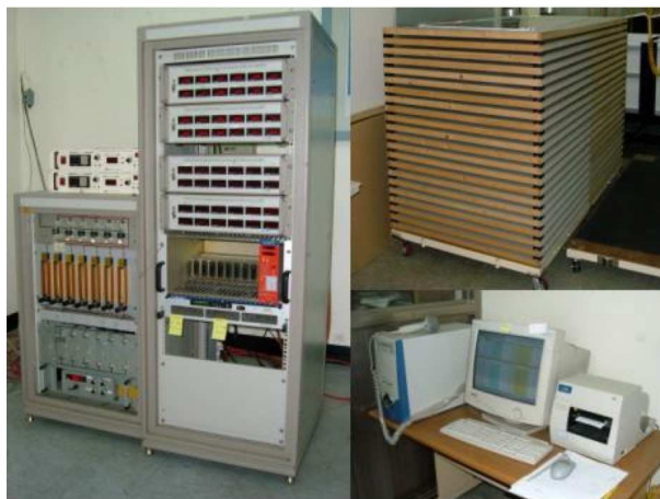
Figure 3.88: Facilities for the high voltage test at Korea University. Three high voltage supplies, four 12-channel current measurement units, and a 6-channel gas supply system are shown on the left panel. The right panel shows 22 RE2/2 full gas gaps for CMS, placed on multi-layer shelves, for the test. After completing the high voltage test, a bar code is assigned to each gas gap for later tracking.
