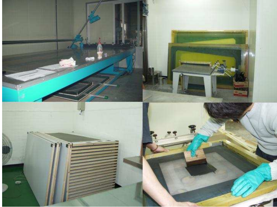
Figure 3.13: Silk screen table and the accessories for the graphite coating. The coating area and the thickness of the carbon layer are controlled by the silk mesh (upper right). The multi-layer shelves (lower left) allow for the drying of the carbon layers for many gaps in parallel. A few samples were made to monitor the variation of the surface resistivity as a function of time (lower right).
