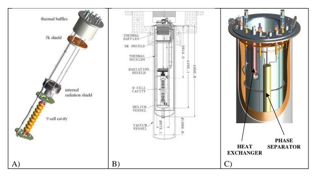
**FIGURE 2.** A) Complete Insert with Cavity; B) Layout of VTS (dimensions in mm) including the dewar, vacuum vessel, insert with cavity; C) Cutaway of cryostat showing heat exchanger and phase separator.
