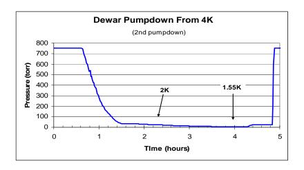
**FIGURE 4**. Initial Pump down of VTS.
