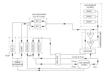
FIGURE 1. IB1 Cryogenic infrastructure and test stand support.
