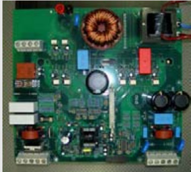
Hardware of PV-Inverter
