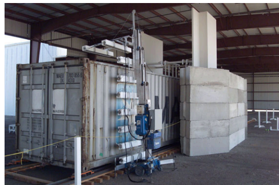
Figure 1. Deployed PPA detector assembly.
