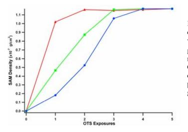
**Figure 2.** Gravimetric C-8 SAM density saturation on microbeads with various diameters, () 10  $\mu$ m, () 20  $\mu$ m, and () 30  $\mu$ m (10 nm pores), resulting from increasing numbers of OTS exposures. SAM saturation density is based on a calculated close-packed SiC<sub>8</sub> density of  $1.17 \times 10^{-7}$  g/cm<sup>2.46</sup>
