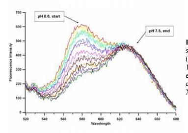
**Figure 7.** Time-dependent fluorescence spectra of SNARF-1-loaded NMsb's (10 μm diameter, 10 nm pores; 1:200-1:250 w/w bR/PL) under 488 nm excitation following consecutive 5 min exposures to a 100 W UV-filtered Xenon lamp.
