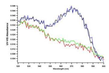
**Figure 3.** Reversible supported bilayer phospholipid exchange with excess SUVs. (red line) SUV exposure (1), PC with 0% mol/mol Rhodamine DHPE. (blue line) SUV exposure (2), PC with 1% mol/mol Rhodamine DHPE. (green line) SUV exposure (3), PC with 0% mol/mol Rhodamine DHPE. (black line) SUV exposure (4), PC with 1% mol/mol Rhodamine DHPE.
