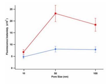
Figure 4. Relative surface areas of (■) EPC and (•) DPPC (each with 0.5% mol/mol Rhodamine DHPE) bilayers on 10 µm beads with varying pore structure. Fluorescence intensities are corrected for the EPC fluid-phase head group area versus the DPPC gel-phase head group area.
