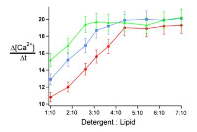
Figure 5. Supported bilayer detergent saturation for various bead diameters measured as calcium release: ( $\bigstar$ ) 10 µm, ( $\blacksquare$ ) 20 µm, and ( $\bullet$ ) 30 µm (10 nm pores). Calcium release was averaged over 1 h after exposure to C12E9. The calculated cmc in this experiment is coincident with 0.08 C12E9/EPC mol/mol.
