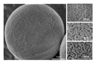
**Figure 1.** SEM images of silica microspheres with varying surface structure. Left:  $10,000 \times$  image of a 10 µm bead with 10 nm pores. Right, descending vertically:  $200,000 \times$  images of beads with 10 nm pores and  $100,000 \times$  images of beads with 50 and 100 nm pores.
