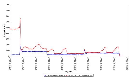
Figure 22. Energy consumed by the OASys unit and furnace AH fan for early September
