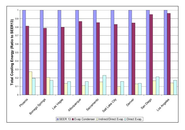
Figure 11. Comparison of four cooling systems in various locations
