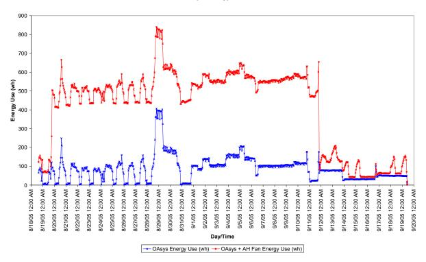
Figure 18. Energy use for OASys and OASys plus furnace AH fan
