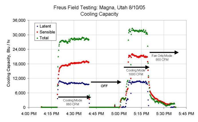
Figure 29. Measurements taken at Magna, Utah, showing the sensible, latent, and total cooling capacities of the Freus unit at two different fans speeds on August 10, 2005
