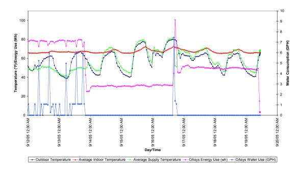
Figure 21. Performance during cool outdoor air temperatures
