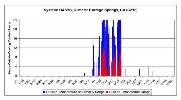
Figure 8. Distribution of hours when indoor temperature or humidity are too high for OASys unit in Borrego Springs, California
