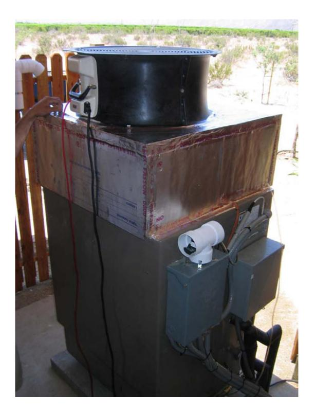
Figure 28. Fan-assisted flow hood installed on the Freus unit
