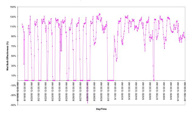
Figure 19. Wet-bulb effectiveness for the OASys unit at Magna
