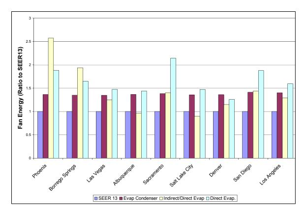
Figure 12. Comparison of fan energy use for cooling systems in various locations
