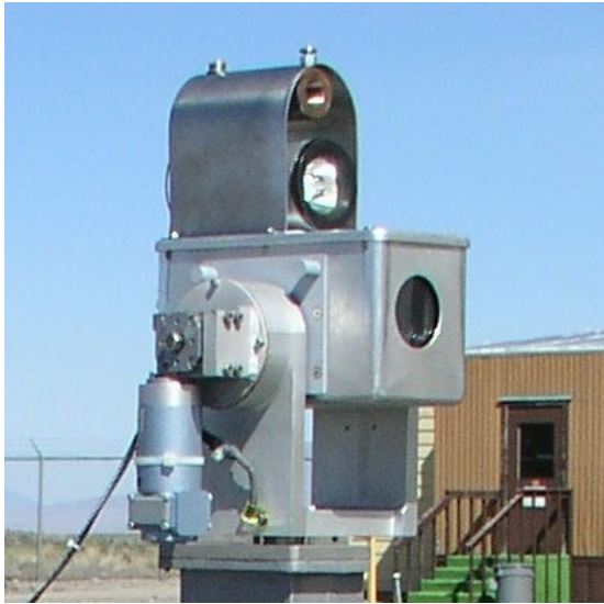
Fig. 1. Proof-of-concept collimated gamma detector. generally possible, aggravated by the tilt motor’s inability to smoothly manipulate the mass of the shielded assembly and its moment as well. The significance of the Table 1 data is in the last row where the smaller source, A (0.8Ci 137Cs), seemingly produces a higher count rate than source B (2.5Ci 137Cs). This anomaly was immediately attributed to insufficient shielding on the sides and bottom of the detector and the testing was halted.
