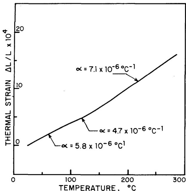
Fig. 6. Linear thermal expansion of a microlitic andesite specimen.
