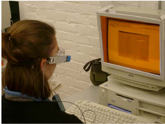
Figure 1: Subject wearing the unfiltered Daysimeter, accompanied by the orange filter on the monitor.
