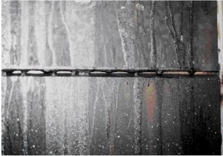
Exhibit 11-56 Photograph of Two Monofrax M Tiles after 35 hr of Coal Firing
