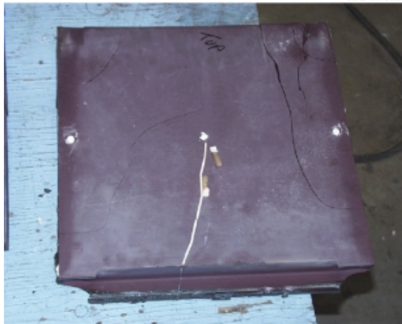
Exhibit 11-66 Photographs of Large Upper Kyocera Tile Before and After SFS Test SFS-RH13-0400
