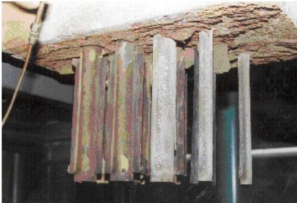
Exhibit 11-54 Photographs of Ash Deposits on the CAH Tubes Following SFS Test SFS-RH13-0400 Firing Eastern Kentucky Bituminous Coals
