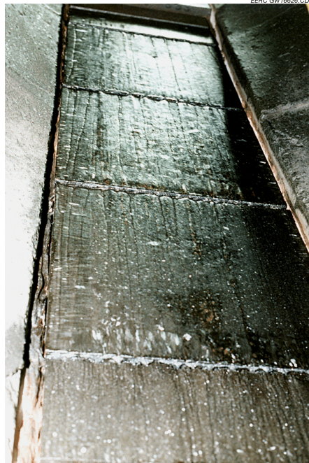
Exhibit 11-62 Photograph of the Monofrax M Tiles from Inside the Furnace Following SFS Test SFS-RH8-0399
