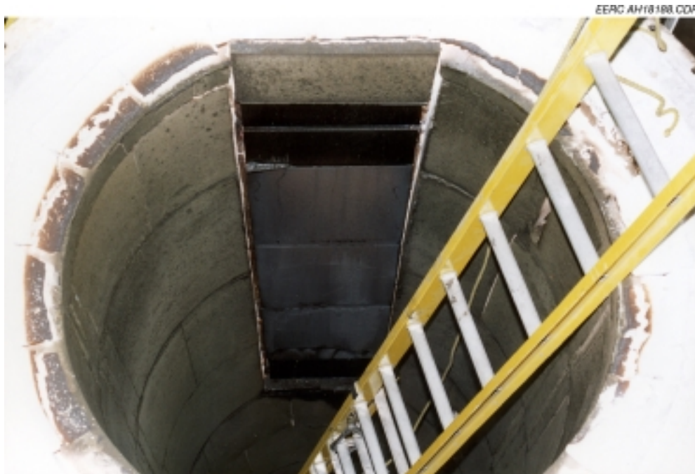
Exhibit 11-65 Photographs of RAH Tiles Before and After SFS Test SFS-RH13-0400
