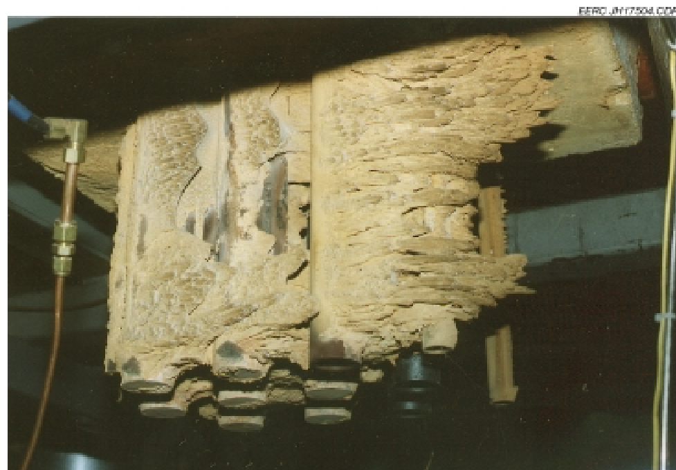
Exhibit 11-45 Photographs of Ash Deposits on the CAH Tubes Following the March 2000 Test Firing Cordero Rojo Subbituminous Coal
