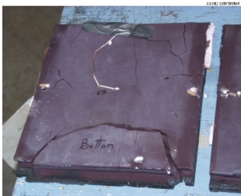
Exhibit 11-68 Photographs of Large Lower Kyocera Tile Before and After SFS Test SFS-RH13-0400
