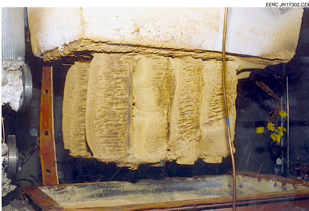
Exhibit 11-36 Photograph of Ash Deposits on the CAH Tubes Following SFS Test SFS- RH11-0799 Firing Illinois No. 6 Bituminous Coal
