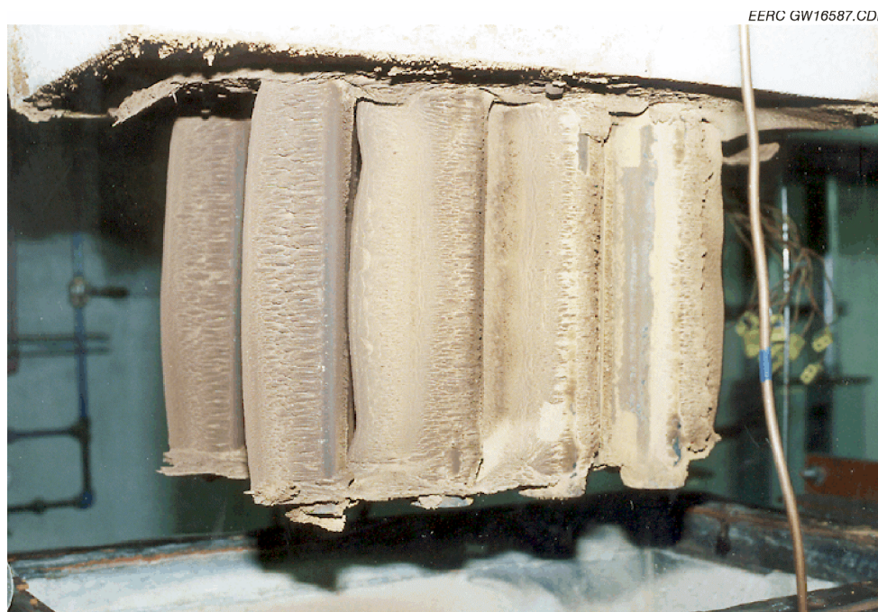
Exhibit 11-51 Photograph of Ash Deposits on the CAH Tubes Following SFS Test SFS-RH8-0399 Firing Eastern Kentucky and Illinois No. 6 Bituminous Coal
