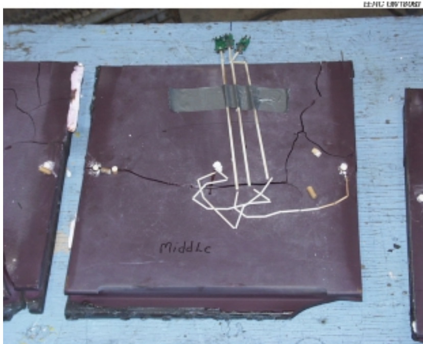
Exhibit 11-67 Photographs of Large Center Kyocera Tile Before and After SFS Test SFS-RH13-0400
