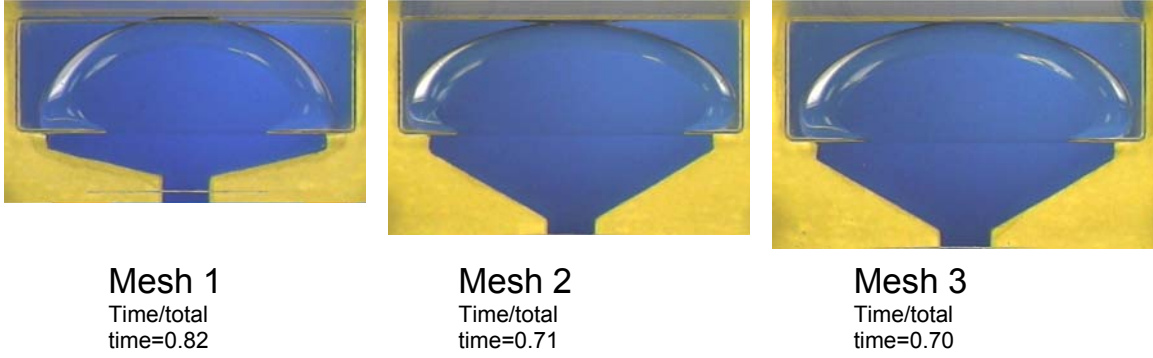
Figure 28. Comparison of the effect of distributor geometry on the time it takes to reach the wall farthest from the injection port in a horizontal orientation.
