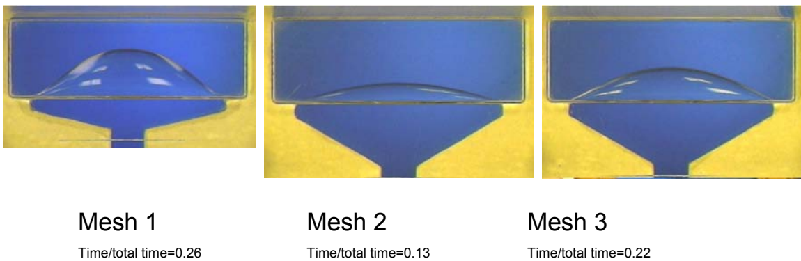
Figure 27. Comparison of the effect of distributor geometry on the shape of the fluid front entering the mold in a horizontal orientation.
