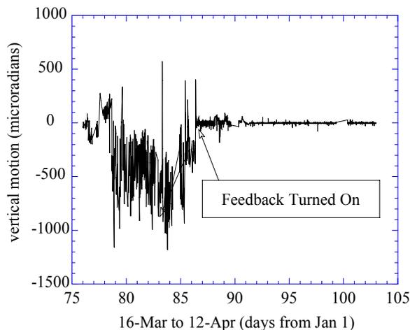
Figure 7. Signal from trajectory stabilization feedback.
