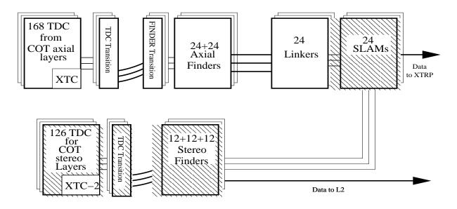
Figure 1. Schematic diagram of the XFT system architecture. The white boxes indicate the original axial system, and the shaded boxes depict the new components introduced with the upgrade. The new Stereo Linker Association Modules (SLAMs) replace the Linker Output Modules (LOMs), which are not shown.
