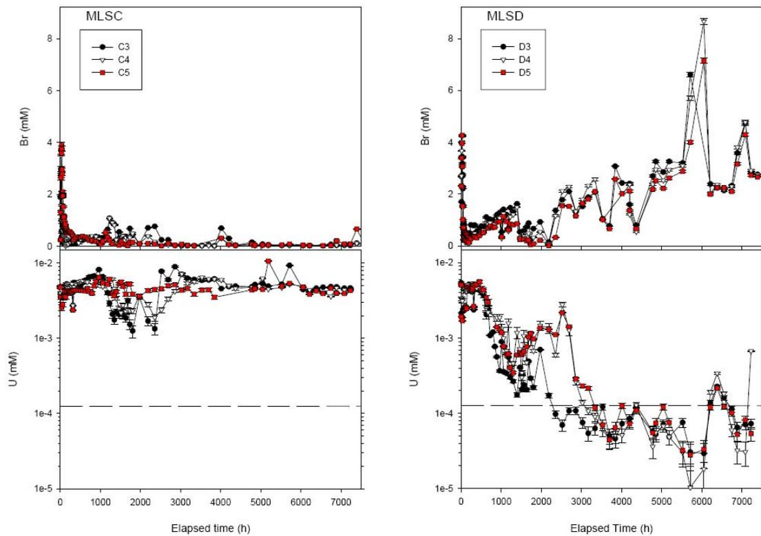
**Figure 2** Bromide (upper panel) and uranium (lower panel) concentrations at multi-level samplers MLSC (left) and MLSD (right) over the entire biostimulation period (eleven months). The dashed line indicates the drinking water standard for dissolved uranium.
