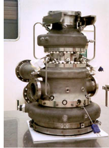
Figure 3-14. Rocket Engine Turbopump (Courtesy of Barber Nichols)
