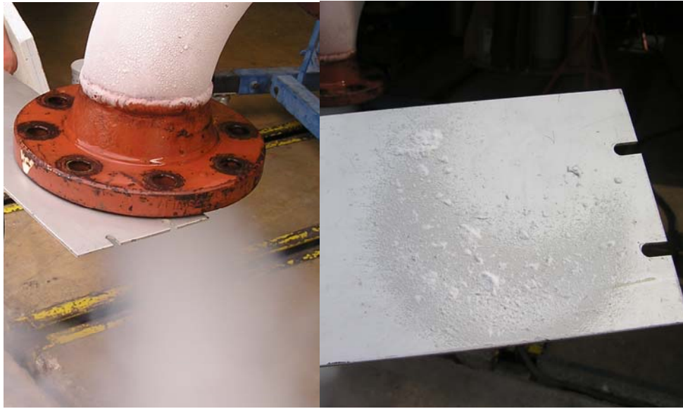
Figure 3-42. Precipitation of H 2 O on Aluminum Plate
