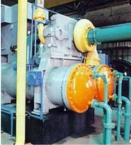
Figure 3-13. Dresser-Rand ISOPAC Compressor (Courtesy of Dresser-Rand)
