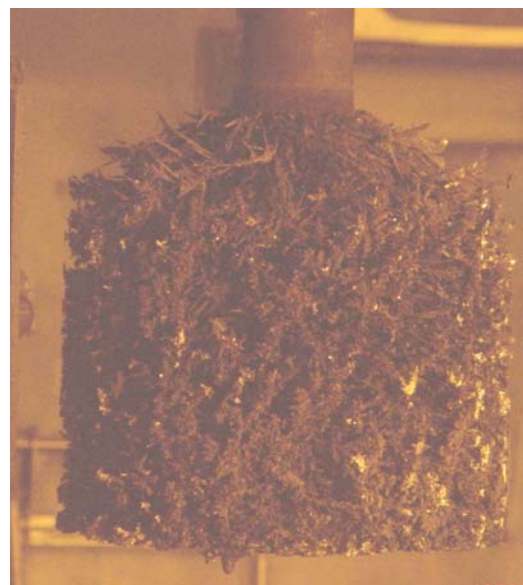
Figure 3. A cathode removed from Mk-IV ER, 10.1 kg
