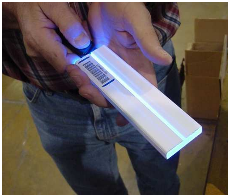
Figure 4.6: Scintillator strips with the WLS fiber.
