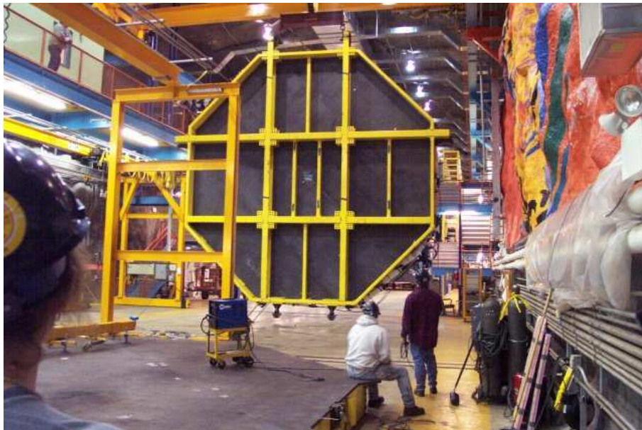
Figure 4.11: A strongback carrying a completed plane.
