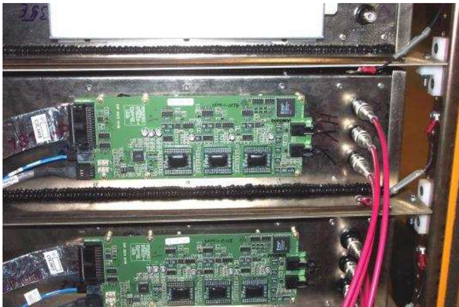
Figure 4.14: A Far Detector Front End Electronics (FEE) board.
