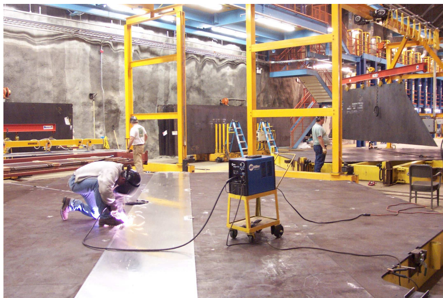
Figure 4.3: Construction of the MINOS Far Detector, two adjacent planes. The Southern plane is in the steel lamination phase, the Northern station has finished its steel lamination and welding phase and has begun to have its first scintillator module welded in place.
